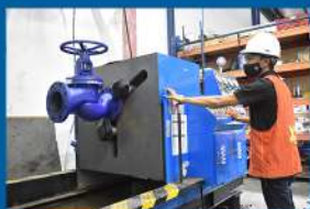
LEAKAGE AND PRESSURE TEST
